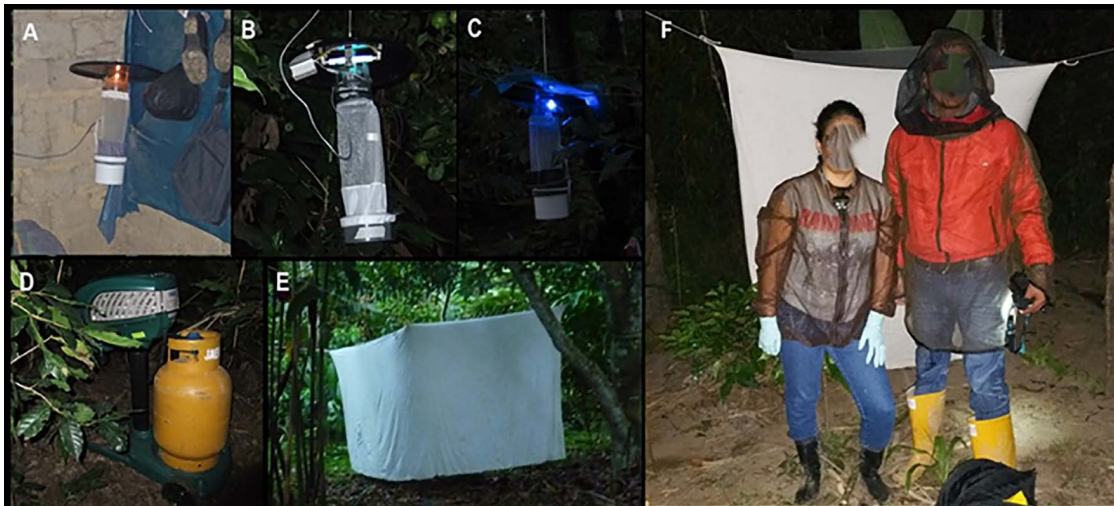
Fig 2. Trap types used for phlebotomine sand fly collections. A) Mini CDC light trap model 512; B) CDC blacklight UV trap model 1212; C) Mini CDC blue LED; D) Mosquito Magnet model Independence baited with CO 2 and R-Octenol; E) Shannon trap; F) protected human landing collection (Photos: VZ).
