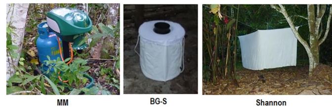
Fig 2. Different trap types used for sand fly collections. LED colors were adapted from the standard Mini CDC light trap Model 512 (CDC). MM: Mosquito Magnet Model Independence baited with CO 2 and R-Octenol; BG-S: BioGents BG Sentinel baited with BG-Lure.
